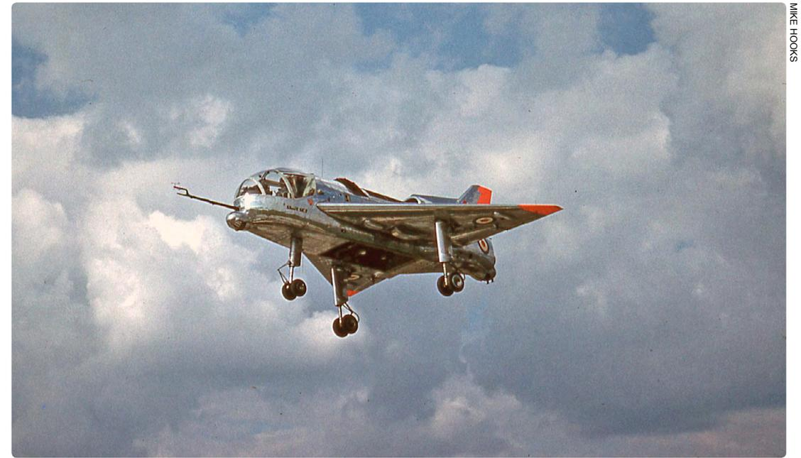
**ABOVE** Shorts designed and built two prototypes — XG900 and XG905 — of the S.C.1 experimental jet-powered vertical take-off and landing (VTOL) aircraft, fitted with four vertical-lift engines and one horizontally mounted for conventional flight. Both had completed transitional flights from vertical to horizontal flight by the end of 1960.
