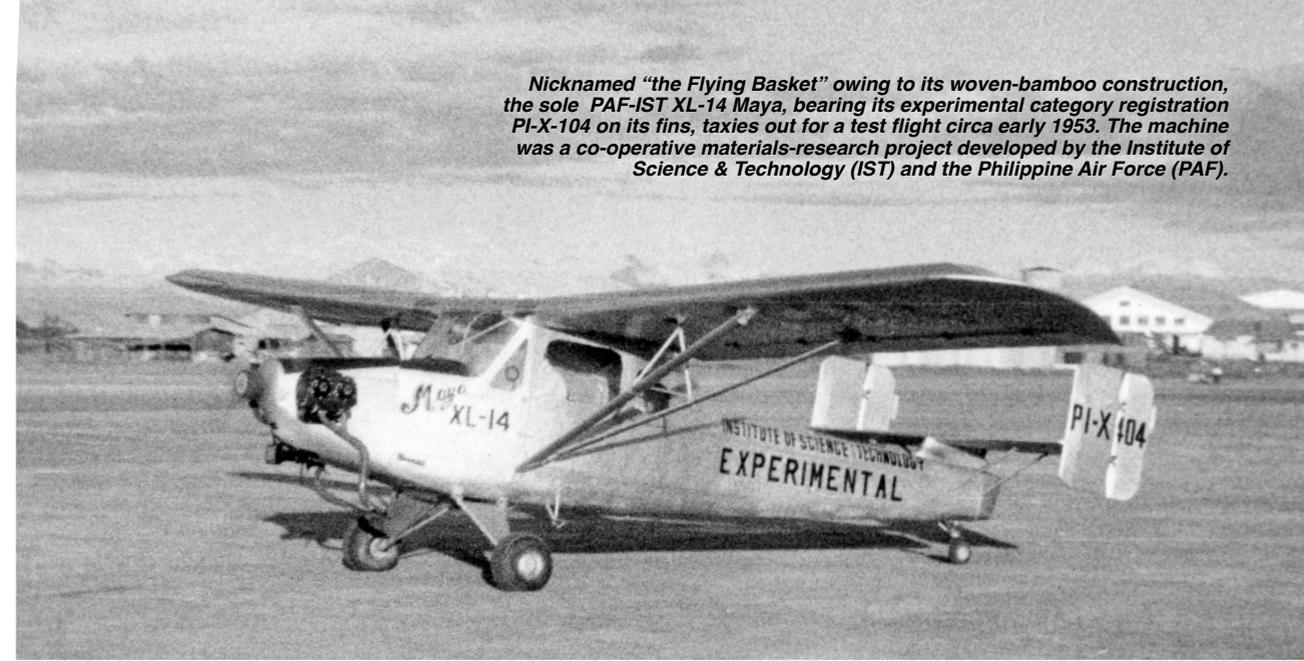
Nicknamed “the Flying Basket” owing to its woven-bamboo construction, the sole PAF-IST XL-14 Maya, bearing its experimental category registration PI-X-104 on its fins, taxis out for a test flight circa early 1953. The machine was a co-operative materials-research project developed by the Institute of Science & Technology (IST) and the Philippine Air Force (PAF).
