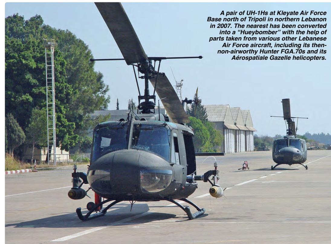
*A pair of UH-1Hs at Kleyate Air Force Base north of Tripoli in northern Lebanon in 2007. The nearest has been converted into a "Hueybomber" with the help of parts taken from various other Lebanese Air Force aircraft, including its then-non-airworthy Hunter FGA.70s and its Aérospatiale Gazelle helicopters.*
