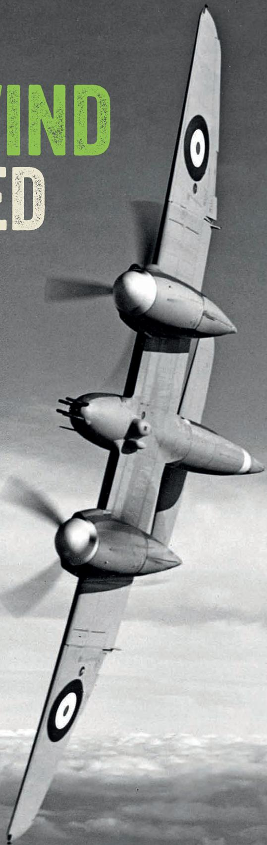
The second prototype Whirlwind, L6845, was tested with propellers of a one-off Rotol design, as seen fitted here. The first prototype, L6844, had been fitted with "handed" Peregrines driving de Havilland propellers, but the props of L6845 rotated in the same direction, the two aircraft sharing broadly similar handling characteristics.
